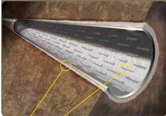
FILTER CAKE IS A BARRIER TO PRODUCTION
