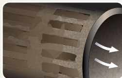
WELLBORE FACE & SCREEN BLOCKED WITH MUD
